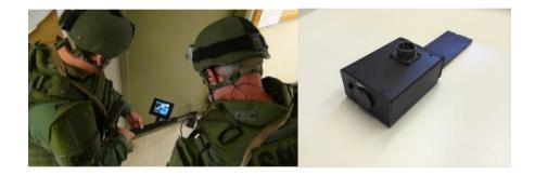
The UDC is used in conjunction with the EyePole, and is interchangeable with the standard surveillance camera that is provided with every EyePole.
